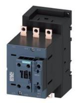
contactor AC-1, 160 A, 690 V / 40 °C, 3-pole, 24 V DC, 0.8-1.2\* Us, with integrated varistor, auxiliary contacts: 1 NO + 1 NC, main circuit: ring cable lug connection, control and auxiliary circuit: screw terminal, size: S3, customer-specific, only expandable with auxiliary switch 3RH2911-2XF22-0KS
