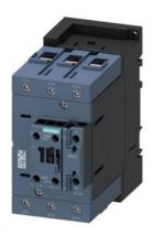
contactor AC-1, 160 A, 690 V / 40 °C, 3-pole, 20-33 V AC/DC, 50/60 Hz, with integrated varistor, auxiliary contacts: 1 NO + 1 NC, main circuit: box terminal, control and auxiliary circuit: screw terminal size: S3
