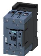
contactor AC-1, 160 A, 690 V / 40 °C, 3-pole, 24 V AC, 50 Hz, auxiliary contacts: 1 NO + 1 NC, main circuit: box terminal, control and auxiliary circuit: screw terminal, size: S3
