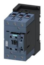
contactor AC-1, 140 A, 690 V / 40 °C, 3-pole, 48-80 V AC/DC, 50/60 Hz, with integrated varistor, auxiliary contacts: 1 NO + 1 NC, main circuit: box terminal, control and auxiliary circuit: screw terminal size: S3
