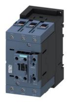
contactor AC-1, 140 A, 690 V / 40 °C, 3-pole, 230 V AC, 50 Hz, auxiliary contacts: 1 NO + 1 NC, main circuit: box terminal, control and auxiliary circuit: screw terminal, size: S3
