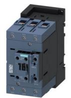
contactor AC-1, 140 A, 690 V / 40 °C, 3-pole, 110 V AC, 50 Hz, auxiliary contacts: 1 NO + 1 NC, main circuit: box terminal, control and auxiliary circuit: screw terminal, size: S3
