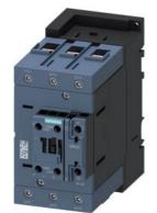
contactor AC-1, 140 A, 690 V / 40 °C, 3-pole, 42 V AC, 50 Hz, auxiliary contacts: 1 NO + 1 NC, main circuit: box terminal, control and auxiliary circuit: screw terminal, size: S3
