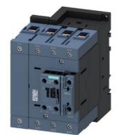
contactor AC-1, 160 A, 400 V / 40 °C, 4-pole, 20-33 V AC/DC, 50/60 Hz, with integrated varistor, auxiliary contacts: 1 NO + 1 NC, screw terminal, size: S3
