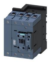
contactor AC-1, 140 A, 400 V / 40 °C, 4-pole, 220 V AC, 50 Hz / 240 V, 60 Hz, auxiliary contacts: 1 NO + 1 NC, screw terminal, size: S3
