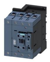
contactor AC-1, 140 A, 400 V / 40 °C, 4-pole, 200 V AC, 50 Hz / 200-220 V, 60 Hz, auxiliary contacts: 1 NO + 1 NC, screw terminal, size: S3
