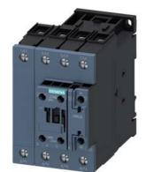
contactor AC-1, 110 A, 400 V / 40 °C, 4-pole, 175-280 V AC/DC, 50/60 Hz, with integrated varistor, auxiliary contacts: 1 NO + 1 NC, screw terminal, size: S2
