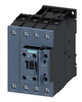
contactor AC-1, 110 A, 400 V / 40 °C, 4-pole, 20-33 V AC/DC, 50/60 Hz, with integrated varistor, auxiliary contacts: 1 NO + 1 NC, screw terminal, size: S2
