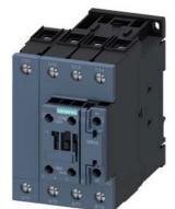
contactor AC-1, 110 A, 400 V / 40  $^\circ$ C, 4-pole, 24 V AC, 50 Hz, auxiliary contacts: 1 NO + 1 NC, screw terminal, size: S2
