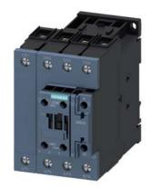
contactor AC-1, 60 A, 400 V / 40 °C, 4-pole, 20-33 V AC/DC, 50/60 Hz, with integrated varistor, auxiliary contacts: 1 NO + 1 NC, screw terminal, size: S2
