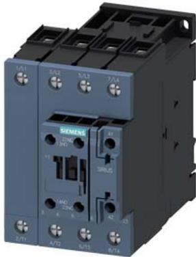
power contactor, AC-3, 51 A, 22 kW / 400 V, 4-pole, 20-33 V AC/DC, 50/60 Hz, with integrated varistor, auxiliary contacts: 1 NO + 1 NC, screw terminal, size: S2
