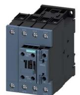
contactor AC-1, 60 A, 400 V / 40  $^\circ$ C, 4-pole, 400 V AC, 50 Hz, auxiliary contacts: 1 NO + 1 NC, screw terminal, size: S2
