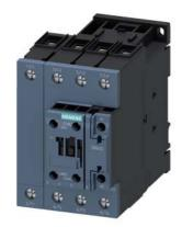
contactor AC-1, 60 A, 400 V / 40 °C, 4-pole, 220 V AC, 50/60 Hz, auxiliary contacts: 1 NO + 1 NC, screw terminal, size: S2
