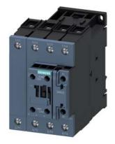
contactor AC-1, 60 A, 400 V / 40 °C, 4-pole, 48 V AC, 50/60 Hz, auxiliary contacts: 1 NO + 1 NC, screw terminal, size: S2
