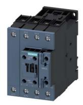
contactor AC-1, 60 A, 400 V / 40 °C, 4-pole, 24 V AC, 50/60 Hz, auxiliary contacts: 1 NO + 1 NC, screw terminal, size: S2
