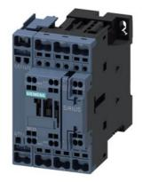
contactor AC-1, 50 A, 400 V / 40 °C, 4-pole, 220 V DC, auxiliary contacts: 1 NO + 1 NC, spring-loaded terminal, size: S0
