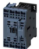
contactor AC-1, 50 A, 400 V / 40 °C, 4-pole, 220 V AC, 50 Hz / 240 V, 60 Hz, auxiliary contacts: 1 NO + 1 NC, spring-loaded terminal, size: S0
