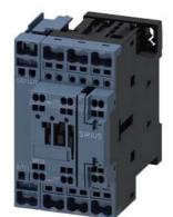
contactor AC-1, 50 A, 400 V / 40 °C, 4-pole, 230 V AC, 50/60 Hz, auxiliary contacts: 1 NO + 1 NC, spring-loaded terminal, size: S0
