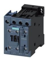
contactor AC-1, 50 A, 400 V / 40 °C, 4-pole, 125 V DC, auxiliary contacts: 1 NO + 1 NC, screw terminal, size: S0
