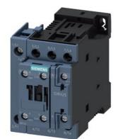
contactor AC-1, 50 A, 400 V / 40 °C, 4-pole, 24 V DC, auxiliary contacts: 1 NO + 1 NC, screw terminal, size: S0
