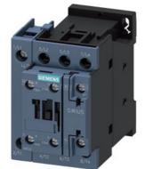
contactor AC-1, 50 A, 400 V / 40 °C, 4-pole, 220 V AC, 50 Hz / 240 V, 60 Hz, auxiliary contacts: 1 NO + 1 NC, screw terminal, size: S0
