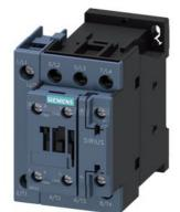
contactor AC-1, 50 A, 400 V / 40 °C, 4-pole, 230 V AC, 50 Hz, auxiliary contacts: 1 NO + 1 NC, screw terminal, size: S0
