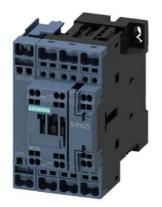
contactor AC-1, 40 A, 400 V / 40 °C, 4-pole, 220 V DC, auxiliary contacts: 1 NO + 1 NC, spring-loaded terminal, size: S0
