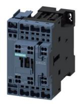
contactor AC-1, 40 A, 400 V / 40 °C, 4-pole, 24 V DC, auxiliary contacts: 1 NO + 1 NC, spring-loaded terminal, size: S0
