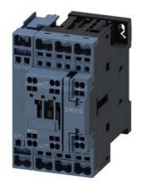
contactor AC-1, 40 A, 400 V / 40  $^{\circ}$ C, 4-pole, 110 V AC, 50 Hz, auxiliary contacts: 1 NO + 1 NC, spring-loaded terminal, size: S0
