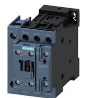
contactor AC-1, 40 A, 400 V / 40  $^\circ\text{C},$  4-pole, 110 V DC, auxiliary contacts: 1 NO + 1 NC, screw terminal, size: S0
