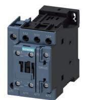
contactor AC-1, 40 A, 400 V / 40  $^{\circ}\text{C},$  4-pole, 24 V DC, auxiliary contacts: 1 NO + 1 NC, screw terminal, size: S0
