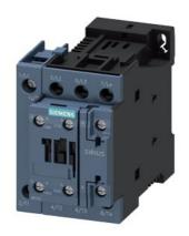
power contactor, AC-3, 32 A, 15 kW / 400 V, 4-pole, 24 V DC, auxiliary contacts: 1 NO + 1 NC, screw terminal, size: S0  $\,$
