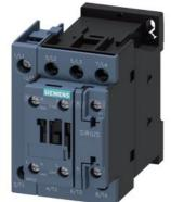
contactor AC-1, 40 A, 400 V / 40 °C, 4-pole, 220 V AC, 50/60 Hz, auxiliary contacts: 1 NO + 1 NC, screw terminal, size: S0
