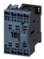
contactor AC-1, 35 A, 400 V / 40 °C, 4-pole, 110 V AC, 50 Hz / 120 V, 60 Hz, with plugged-in varistor, auxiliary contacts: 1 NO + 1 NC, spring-loaded terminal, size: S0
