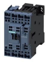
contactor AC-1, 35 A, 400 V / 40 °C, 4-pole, 220 V DC, auxiliary contacts: 1 NO + 1 NC, spring-loaded terminal, size: S0
