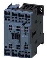
contactor AC-1, 35 A, 400 V / 40 °C, 4-pole, 230 V AC, 50/60 Hz, auxiliary contacts: 1 NO + 1 NC, spring-loaded terminal, size: S0
