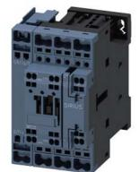
contactor AC-1, 35 A, 400 V / 40 °C, 4-pole, 110 V AC, 50 Hz / 120 V, 60 Hz, auxiliary contacts: 1 NO + 1 NC, spring-loaded terminal, size: S0
