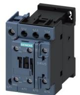
contactor AC-1, 35 A, 400 V / 40  $^\circ$ C, 4-pole, 24 V AC, 50 Hz, auxiliary contacts: 1 NO + 1 NC, screw terminal, size: S0
