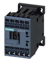
contactor AC-1, 22 A, 400 V / 40  $^\circ\text{C},$  4-pole, 208 V AC, 50/60 Hz, spring-loaded terminal, size: S00
