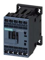
contactor AC-1, 22 A, 400 V / 40 °C, 4-pole, 48 V AC, 50/60 Hz, spring-loaded terminal, size: S00
