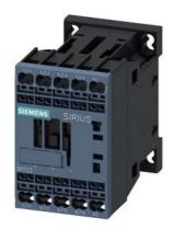
contactor AC-1, 18 A, 400 V / 40  $^{\circ}$ C, 4-pole, 220 V AC, 50 Hz / 240 V, 60 Hz, spring-loaded terminal, size: S00
