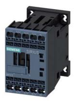
contactor AC-1, 18 A, 400 V / 40 °C, 4-pole, 230 V AC, 50/60 Hz, spring-loaded terminal, size: S00  $\,$
