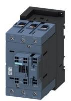
traction contactor, AC-3e/AC-3, 110 A, 55 kW / 400 V, 3-pole, 24 V DC, 0.7-1.25\* Us, electronic drive, with integrated varistor, auxiliary contacts: 1 NO + 1 NC, main circuit: screw terminal, control and auxiliary circuit: spring-loaded terminal, size: S3
