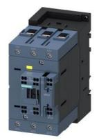
power contactor, AC-3e/AC-3, 110 A, 55 kW / 400 V, 3-pole, 21-33 V AC/DC, 50/60 Hz, with integrated varistor, auxiliary contacts: 1 NC, main circuit: screw terminal, control and auxiliary circuit: spring-loaded terminal, size: S3, F-PLC-IN
