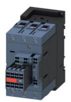
power contactor, AC-3e/AC-3, 110 A, 55 kW / 400 V, 3-pole, 20-33 V AC/DC, 50/60 Hz, with integrated varistor, auxiliary contacts: 2 NO + 2 NC, main circuit: screw terminal, control and auxiliary circuit: spring-loaded terminal, size: S3, captive auxiliary switch
