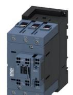
power contactor, AC-3e/AC-3, 110 A, 55 kW / 400 V, 3-pole, 20-33 V AC/DC, 50/60 Hz, with integrated varistor, auxiliary contacts: 1 NO + 1 NC, main circuit: screw terminal, control and auxiliary circuit: spring-loaded terminal, size: S3, communication-capable
