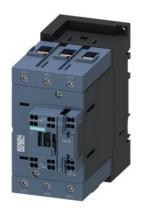
power contactor, AC-3e/AC-3, 110 A, 55 kW / 400 V, 3-pole, 24 V AC, 50 Hz, auxiliary contacts: 1 NO + 1 NC, main circuit: screw terminal, control and auxiliary circuit: spring-loaded terminal, size: S3  $\,$
