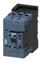
power contactor, AC-3e/AC-3, 110 A, 55 kW / 400 V, 3-pole, 230 V AC, 50 Hz, auxiliary contacts: 1 NO + 1 NC, screw terminal, size: S3, upright mounting position
