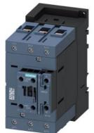
power contactor, AC-3e/AC-3, 110 A, 55 kW / 400 V, 3-pole, 24 V AC, 50 Hz, auxiliary contacts: 1 NO + 1 NC, screw terminal, size: S3, upright mounting position
