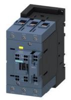
power contactor, AC-3e/AC-3, 95 A, 45 kW / 400 V, 3-pole, 21-33 V AC/DC, 50/60 Hz, with integrated varistor, auxiliary contacts: 1 NC, main circuit: screw terminal, control and auxiliary circuit: spring-loaded terminal, size: S3, F-PLC-IN
